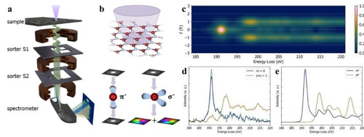
Fig. 1: a) Experimental setup to realize OAM-EELS double dispersion. b) Sketch of electron beam illumination on h-BN at 5.4 mrad and the electron wavefunction after single scattering on boron. c) Experimental OAM-EELS after model-based fitting to remove inelastic delocalization and psf of the sorter. d) experimental EEL spectra for  $|m| = 1$  and (dashed lines are raw results, full lines are smoothed curves). e) Corresponding theoretical spectra.
