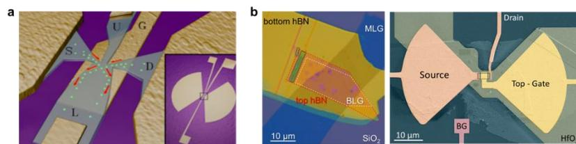
Fig. 1: High-performance terahertz photodetectors. (a) Schematic diagram of a graphene-based ballistic rectifier. (b) Optical and scanning electron micrograph (SEM) images of an antenna coupled tunnel field-effect transistor based on bilayer graphene.
