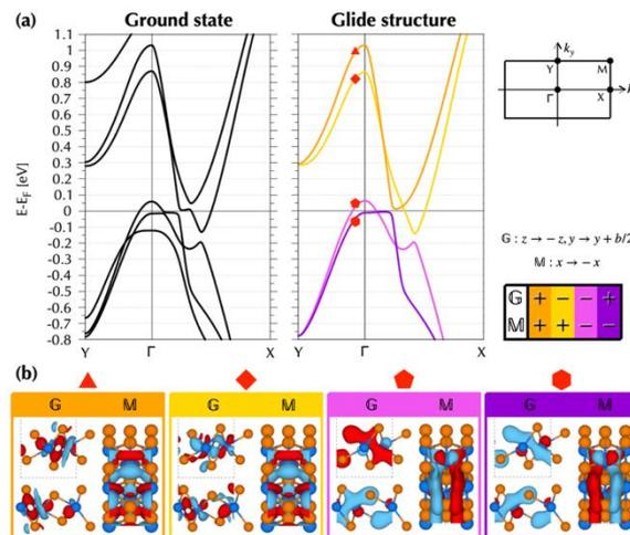
Fig. 1: (a) DFT-PBE bands of bilayer WTe<sub>2</sub>: ground state structure (left) and structure with glide symmetry (right). Brillouin zone in the top right corner. (b) Real part of Kohn-Sham wavefunctions at k points marked by red shapes. The side and top views show the sign of the states with respect to the glide ( $G$ ) and mirror ( $M$ ) symmetry, as reported in the table.
