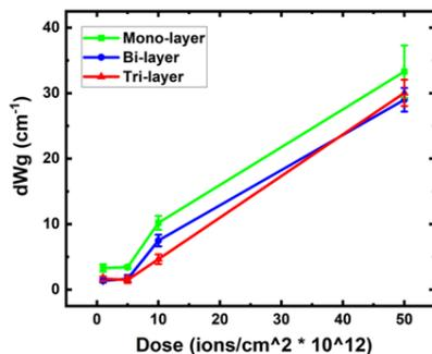
Fig.1: Mono-, bi-, and tri-layer graphene G-peak width change with the different He-ion dose.
