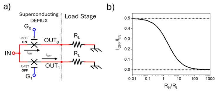
Fig. 2: a) Schematic circuit of a superconducting DEMUX with the load stage. b) Ratio between the current flowing in the OFF and ON branch as a function of  $R_N/R_L$ .
