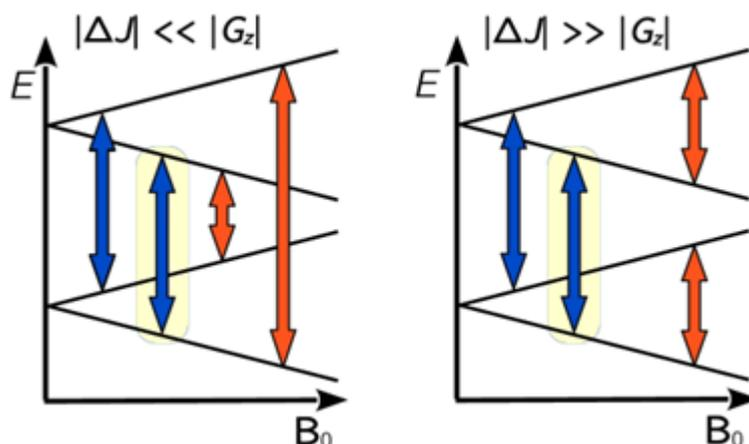
Fig. 1: Schematic representation of the electric-dipole (blue arrows) and magnetic-dipole transitions (red arrows) between the lowest states of the molecular spin triangle. The schemes refer to the limiting cases of a chirality (left) and of an exchange qubit (right), corresponding to an exchange inhomogeneity ( $\Delta J$ ) that is smaller or larger than the Dzyaloshinskii–Moriya interaction ( $G_z$ ), respectively.
