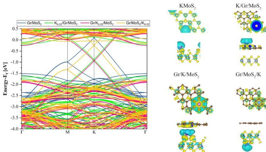
Fig. 1: Band structures and charge density difference plots (isosurface level:  $0.0007e/\text{\AA}^3$ ) of  $\text{KMoS}_2$ ,  $\text{K/Gr/MoS}_2$ ,  $\text{Gr/K/MoS}_2$ , and  $\text{Gr/MoS}_2/\text{K}$ .
