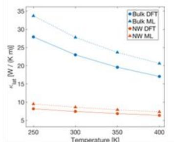
Figure 2. Lattice thermal conductivity calculated with the full approach (labeled DFT) and with
