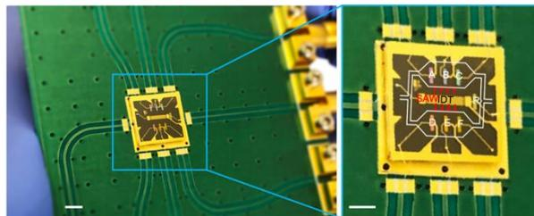
Fig. 1: A complete surface acoustic wave (SAW) biochip featuring six high-frequency resonator biosensors (A–F) and a low-frequency mixing interdigital transducer (SAW-IDT). In the zoomed image on the right, white lines outline the structure of the microfluidic chip layer.
