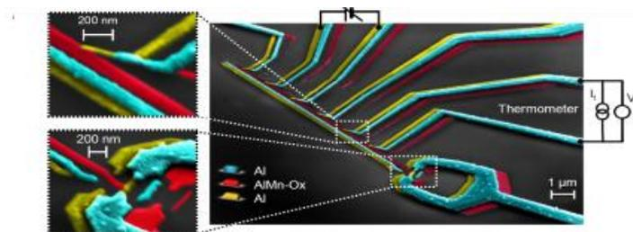
Fig. 1: Thermal superconducting quantum interference proximity transistor.
