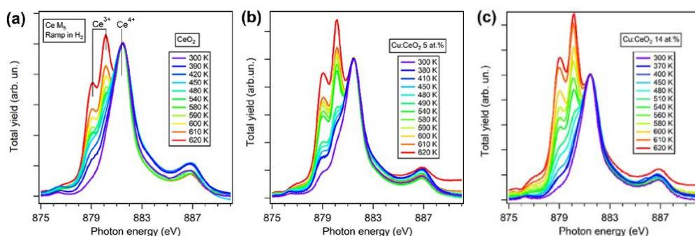
Fig. 1: Ce M<sub>5</sub>-edge XANES spectra of (a) undoped CeO<sub>2</sub> (b) a Cu:CeO<sub>2</sub> 5 at. % doped film and (c) a Cu:CeO<sub>2</sub> 14 at. % doped film acquired at different T in H<sub>2</sub> at ambient pressure
