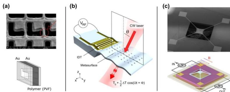
Fig. 1 (a): anisotropic metasurface for studies on the singular value decomposition of the scattering matrix in chiral systems; (b) piezoelectric metasurface for high frequency modulation of laser beams; (c) microbolometric membranes for room-temperature terahertz radiation detectors.
