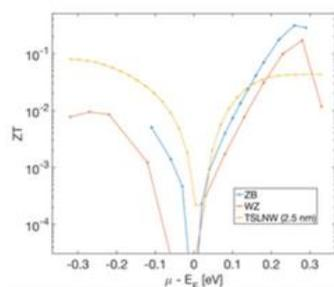
Figure 1. Figure of merit of InAs zincblende (ZB), wurtzite (WZ) and twinned superlattice nanowire with 2.5 nm
