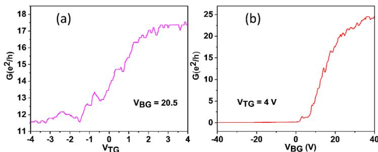
Fig. 1: Conductance modulation in a dual-gated 2D-InSb/Nb-based hybrid Josephson junction: (a) Conductance vs. top gate voltage at a fixed bottom gate voltage of 20.5 V, and (b) conductance vs. bottom gate voltage at a fixed top gate voltage of 4 V, at T = 4 K.
