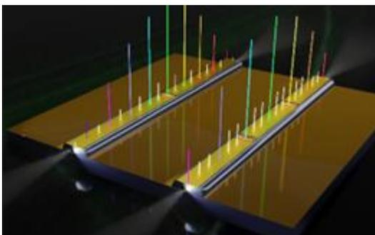
Fig 1: Engineered Fabry-Perot THz harmonic frequency comb with graphene scatters on the metallic top contact, allowing for steady comb emission at a specific harmonic order.
