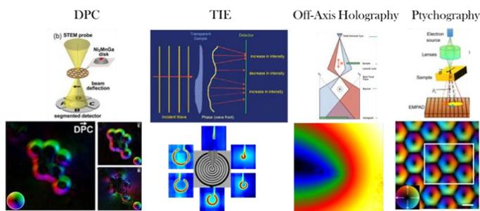
Fig. 1: Schematic representation for the four techniques for phase retrieval. For each technique the top row shows the working principle, while the bottom row shows experimentally retrieved phases. For DPC and Ptychography the experimental phases have been taken from [1] and [5] respectively.
