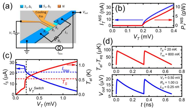
Fig. 1: The QUISTRON is a superconducting nanowire device that generates GHz-range oscillations through thermal cycling. a)
