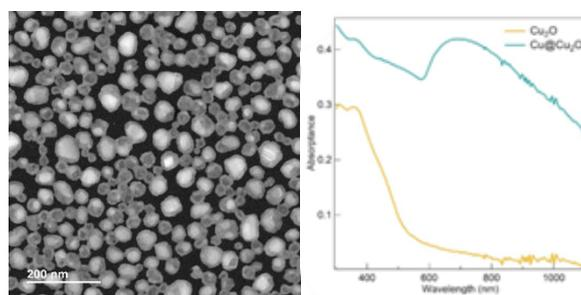
Fig. 1: STEM image of Cu@ $\text{Cu}_2\text{O}$  NPs (left); absorbance spectra which highlight the extended absorption range of Cu@ $\text{Cu}_2\text{O}$  compared to  $\text{Cu}_2\text{O}$  alone (right).
