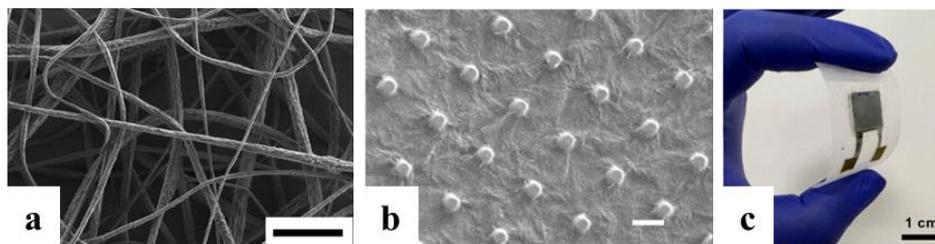
Fig. 1: Scanning electron micrographs of a) random piezoelectric polymer nanofibers (Scale bar: 5  $\mu\text{m}$ ) and b) nanopatterned Cellulose/Polyvinylalcohol composite, planar view (Scale bar: 1  $\mu\text{m}$ ). c) Photograph of a flexible piezoelectric device.
