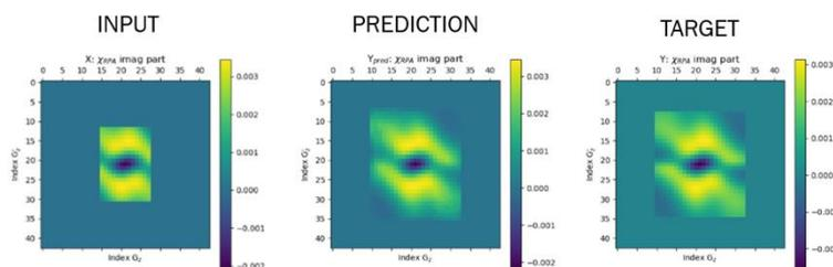
Fig. 1: Example of performance on hBN RPA response slices, trained on hBN independent-particle ones, where X is the input image (4 Ry), Y the target output (8 Ry) and Ypred the prediction.
