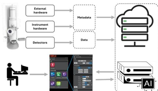
Fig. 1: Schematic of an AI-powered, cloud-integrated TEM workflow: Experimental data and metadata from the TEM, including detectors and external hardware, are transmitted to cloud storage for remote access. Users interact with analysis software, leveraging AI-driven tools for automated data interpretation and decision-making.
