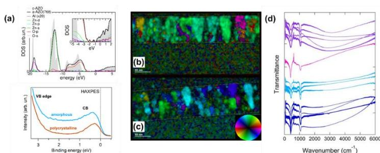
Fig. 1: (a) DFT calculation of DOS and HAXPES measurements on polycrystalline (c-) and amorphous (a-) AZO films; (b,c) FFT analysis of HRTEM images and (d) reflectivity of c- and a-AZO films.
