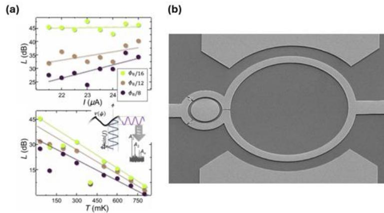
Fig. 1: (a) The linearity of the voltage-flux response of the  $\Phi_0/8$ - $\Phi_0/12$ - $\Phi_0/16$  bi-SQUIDs extracted from the experimental data of ref [1]. (b) Scanning electron micrograph of a double-loop dc superconducting quantum interference device (bi-SQUID) based on Nb superconductor–normal-metal–superconductor ( $\Phi_0/8$ - $\Phi_0/12$ - $\Phi_0/16$ ) proximity Josephson junctions.
