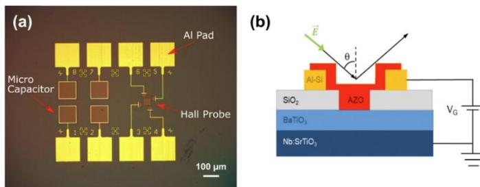
Fig. 1: (a) Microcapacitors fabricated via EBL. (b) Cross-section of the stacking of the layer films.
