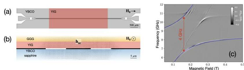
Fig. 1: (a) Top view and (b) section of the YBCO coplanar resonator with the YIG film placed on top. (c) Polariton spectrum acquired at 30 K.
