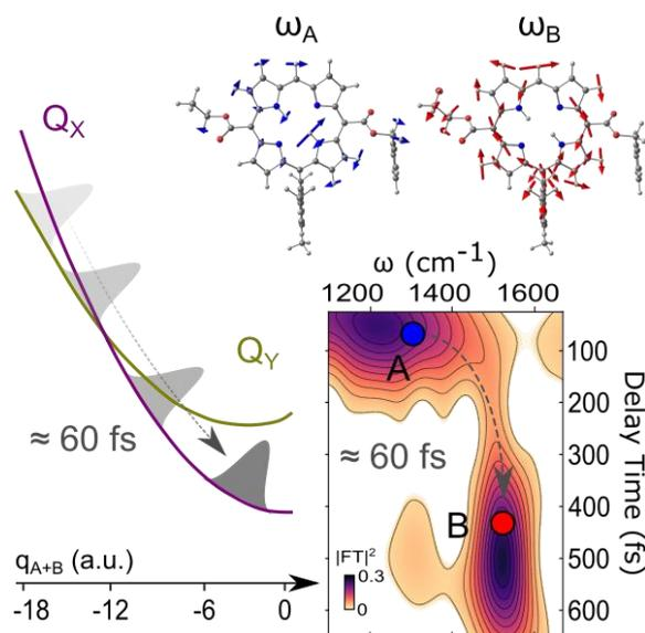
Fig. 1: Internal conversion in a porphyrin derivative proceeds through a crossing of the two Q sub-bands. The vibration modes driving the conversion are theoretically predicted and the ultrafast conversion dynamics is observed via 2D electronic spectroscopy. (from [3]).
