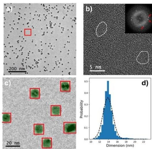
Fig. 1: a) TEM image of Cu NPs on CaF<sub>2</sub> b) HR-TEM acquired in the red-squared region in (a): the small crystals reveal the polycrystalline nature of the CaF<sub>2</sub> film. The inset shows the associated FFT. c) Detection and segmentation of Cu NPs using Mask R-CNN, showing bounding boxes and segmentation masks around individual particles. d) Diameter distribution of Cu NPs obtained from the statistical analysis of 30 TEM images, covering a total of 5392 particles.
