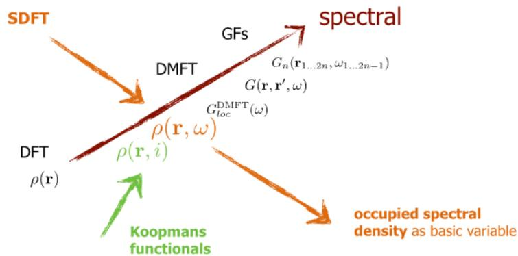
Fig. 1: Climbing the hierarchy of spectral electronic-structure methods: From the charge density to the spectral density as basic variable.
