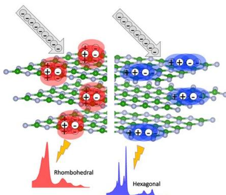
Fig. 1: Schematic representation of exciton-phonon spectroscopy in layered materials in the case of phonon-assisted cathodoluminescence: an electron beam generates excitons in the system, which later radiatively recombine thanks to the mediation of lattice vibrations. The fine structure of the luminescence spectrum depends on the symmetry of the crystal dictating the exciton-phonon selection rules.
