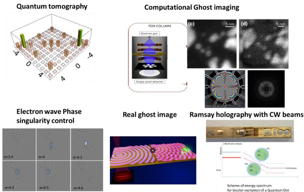
Fig. 1: Some of the directions of quantum developments in our TEM research: a) first quantum state tomography in OAM basis, b) computational ghost imaging c) Control of phase singularities and "Hilbert Hotel" experiments d) real ghost imaging using entanglement e) Ramsay holography and two state interference to measure phase in inelastic scattering.
