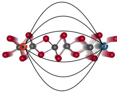
Fig. 1: Schematic representation of electron-hole interaction in WTe<sub>2</sub> monolayer
