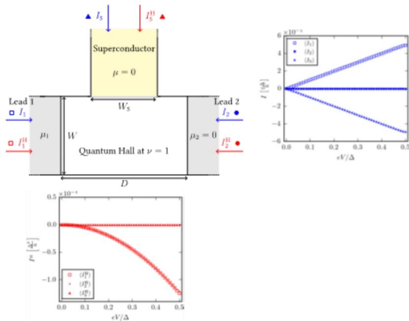
Fig. 1: Quantum Hall/Superconductor setup (left), charge (middle) and heat (right) currents.
