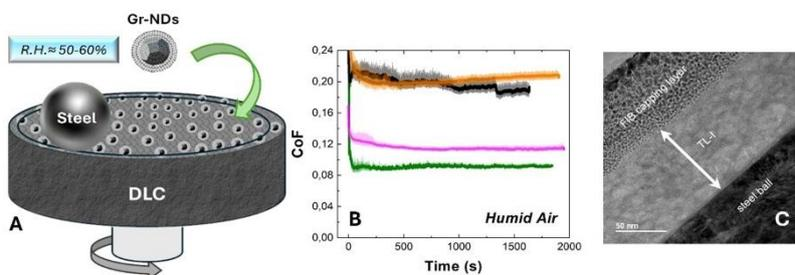
Fig. 1: A) Not-to-scale scheme diagram of tribological test performed in humid environment on DLC substrate functionalized with Graphitic Nanodiamonds (Gr-NDs). B) CoFs plots as a function of time of DLC substrate functionalized through different carbon nanostructures. C) HRTEM image from the cross-sectional sample of the transfer layer.
