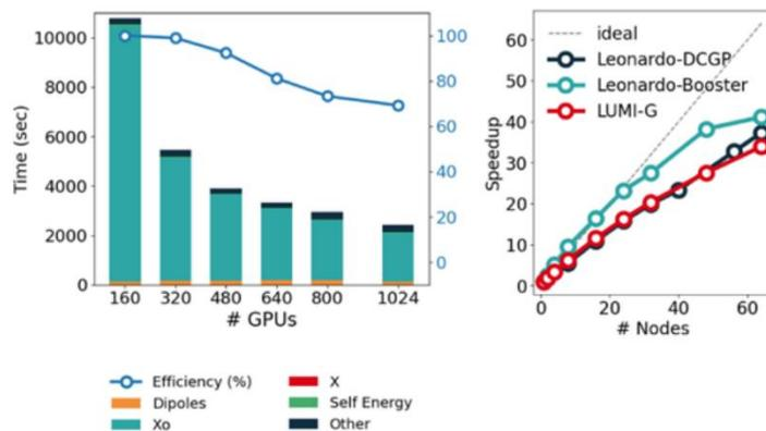
Fig. 1: Calculation of quasi-particle corrections on a graphene/Co interface. On the left, the scalability test on Leonardo-Booster (CINECA), while at the right a speedup comparison between Leonardo-DCGP, Leonardo-Booster and LUMI-G (CSC) for the same system but with reduced parameters.
