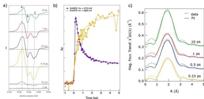
Fig. 1: a) Ce L<sub>3</sub>-edge XANES pump-probe difference spectra at different delay times; b) Kinetic traces of the Ce L<sub>3</sub> edge pump-probe signal in the XANES region at hn=5723 eV (purple) and in the EXAFS region at hn=5825 eV (yellow), with the exponential fits of the signals in the 0-5 ps region; c) Magnitude of the Fourier transform of the k<sup>3</sup>-weighted first-shell Dχ(k) (solid lines) and fits (dashed lines) at different delay times.
