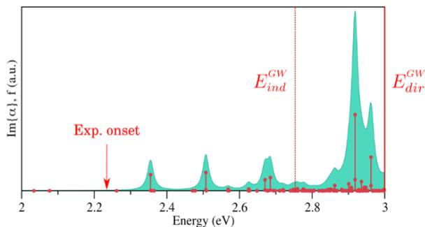
Fig. 1: BSE optical response of monolayer SnS2 for in-plane electric-field polarization: red dots and bars indicate the optical excitation energies and associated oscillator strengths, the light-green curve is the imaginary part of the 2D polarizability, and the vertical lines indicate the direct and indirect GW band gaps. The experimental absorption onset was taken from [1].
