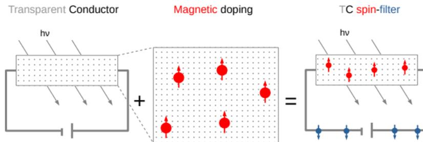
Fig. 1: Graphical representation of the identification of potential transparent conductor spin-filter.
