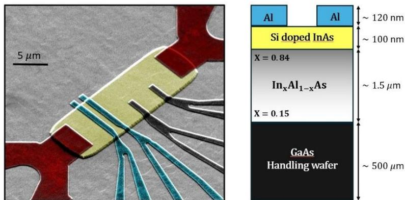
Fig. 1: On the left, a SEM (scanning electron microscopy) image of the device used for the measurements. On the right, a sketch of the InAsOI heterostructure.
