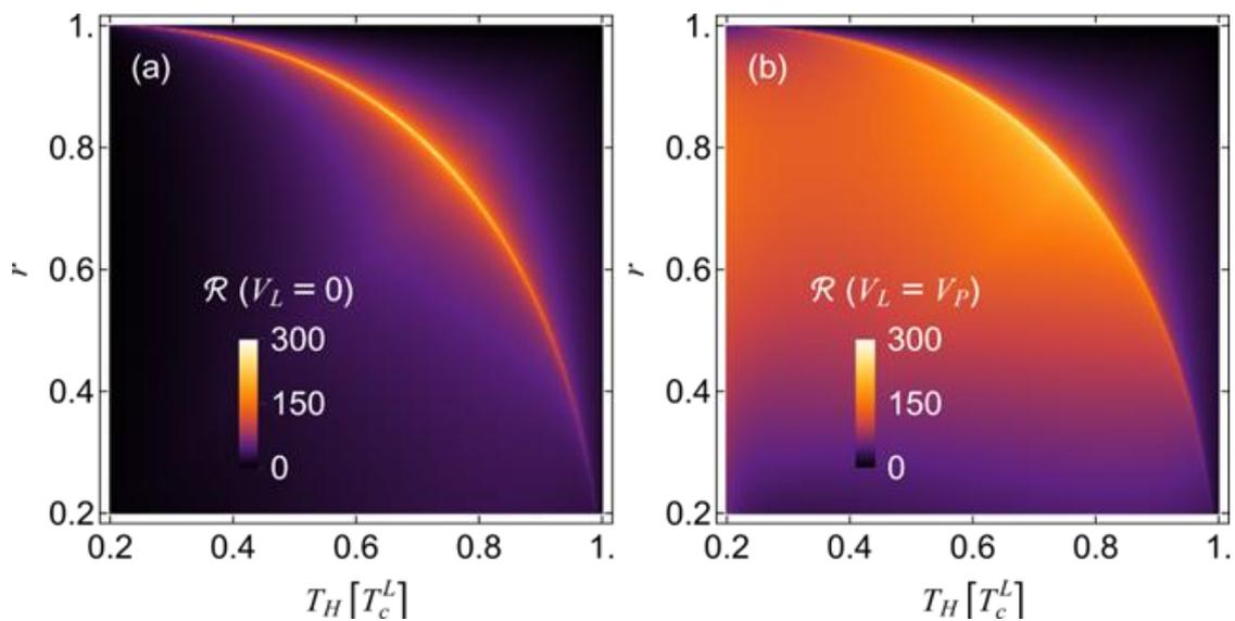
Fig. 1: Rectification efficiency  $\mathcal{R}$  as a function of the hot electrode temperature  $T_H$  and the gap ratio  $r$ , evaluated at an applied voltage  $V_L=0$  in (a) and at the matching peak voltage  $V_L=V_P$  in (b). The matching peak  $V_P$  arises due to the asymmetric superconducting energy gaps, where the ratio  $r$  between the two deviates from unity.
