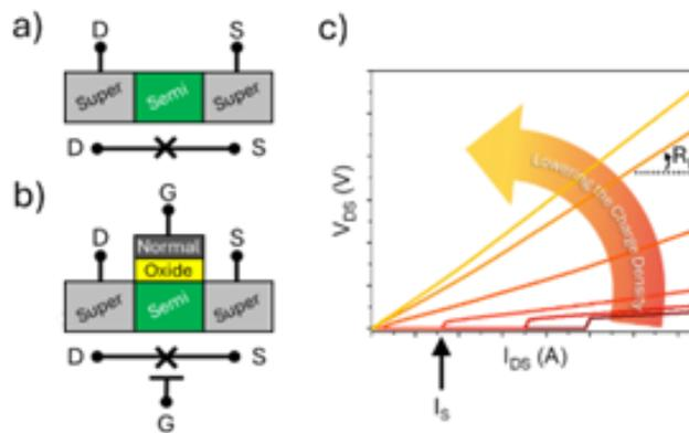
Fig. 1: a,b) The structure and schematic symbols of a JJ (a) and a JoFET (b). c) The  $V_{DS}$  versus  $I_{DS}$  characteristics of a JoFET resulting from the reduction of semiconductor charge density when applying gate voltage.
