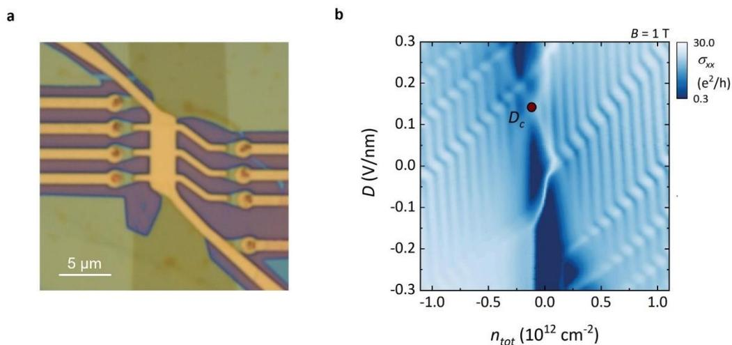
Fig. 1: (a) Optical microscopy image of a dual-gated twisted trilayer device. (b) Longitudinal conductivity at  $B = 1$  T, as a function of charge density ( $n$ ) and displacement field ( $D$ ).  $D_c$  marks the gap closing in the Bernal subsystem.
