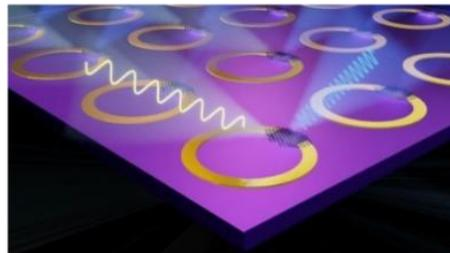
Fig. 1: (a) Schematic diagram of a QCL-pumped graphene split ring resonator array: pumped light is frequency upconverted at the third harmonic frequency. (b) Device schematics of a plasmonic heterostructure laser with an integrated topological insulator stack.
