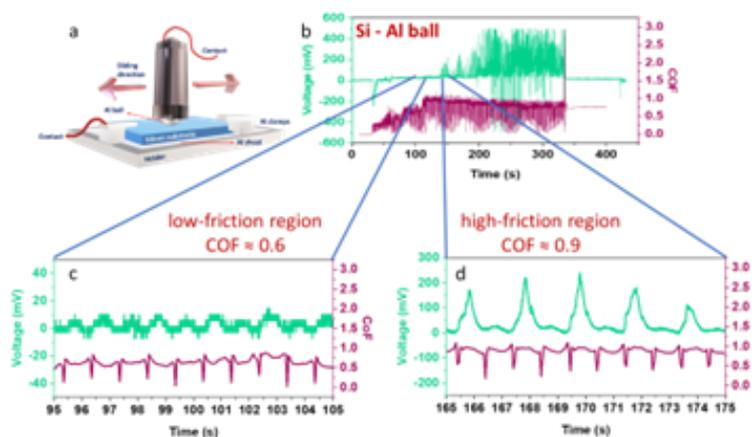
Fig. 1: (a) Representation of the triboelectric setup, (b) Case study of Si-Al pair under an applied load of 20 N and a sliding velocity of 15 mm/s, focused area for (c) low-friction and (d) high-friction regions.
