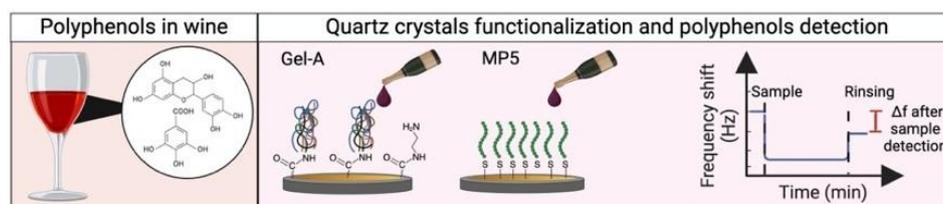
Fig. 1: Chemical functionalization and detection of polyphenols in wines by QCM-D.
