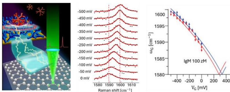
Fig. 1: An opto-electronic graphene-based biosensor detects immunoglobulin M (IgM) at 100 zeptomolar ( $10^{-19}$  M) concentration. It features a biofunctionalized gold electrode capacitively coupled to a graphene electrode via a water-soaked paper strip. Surface potential changes induced by few affinity events are transduced as shifts of the graphene phonon frequencies and detected by Raman spectroscopy.
