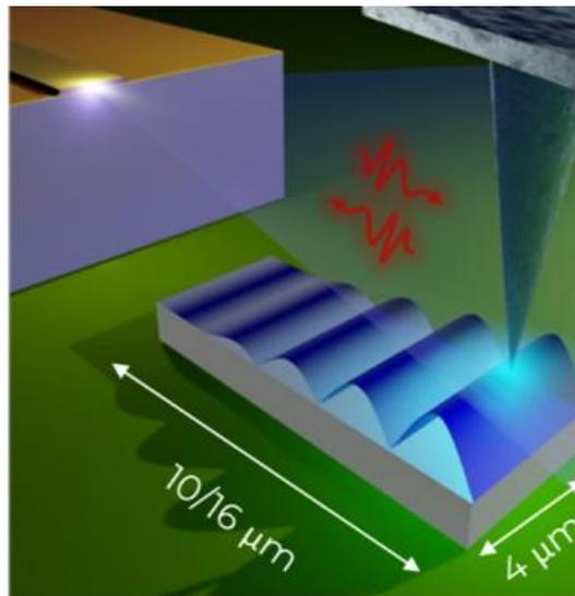
Fig. 1: Schematics of THz Dirac plasmon polaritons (DPPs) of a  $\text{Bi}_2\text{Se}_3$  antenna resonator launched by the s-SNOM tip under excitation with a THz quantum cascade laser (QCL) (adapted from [4]).
