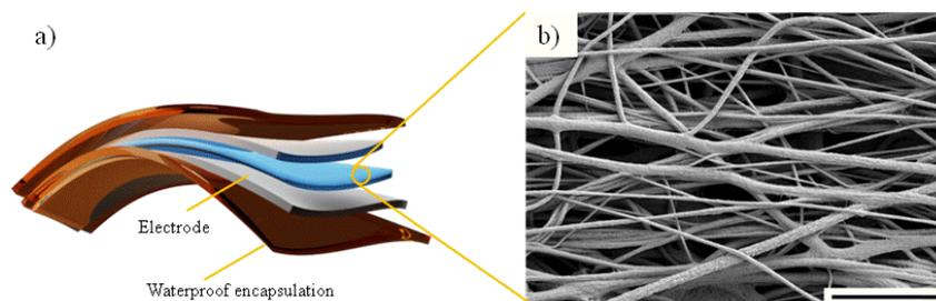
Fig. 1: a) Schematic of the piezoelectric device developed and b) scanning electron micrograph of piezoelectric nanofibers. Scale bar: 10µm.
