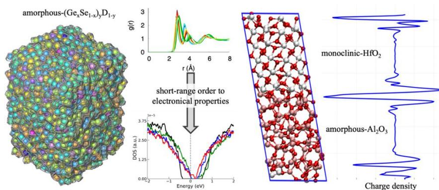
Fig. 1: From left to right: the amorphous structure of doped-GeSe systems colored accordingly to its Voronoi geometry; the radial distribution functions and Density of States; the interface between m-HfO<sub>2</sub>/a-Al<sub>2</sub>O<sub>3</sub> and the charge density across the interface.
