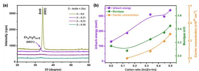
Fig. 1: (a) X-ray diffraction patterns and (b) opto-electrical properties of ITO-ZnO mixed oxides for different cation ratios.
