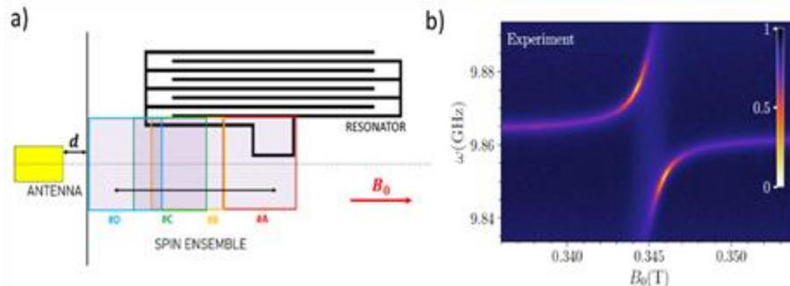
Fig. 1: a) Sketch of the microwave resonator coupled to its feeding antenna and with four sample positions (#A to #D) used in experiments. b) Reflection map showing the polaritons and the dips at which Perfect Absorption Occurs.
