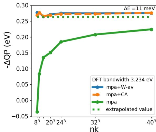
Fig. 1: QP correction to the bandwidth of a 3D metal bulk Na with respect to the number of points in the k-grid, computed with (blue line) and without (green line) the W-av method.
