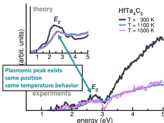
Fig. 1: Comparison between experimental and theoretical (inset) EELS spectra of high entropy HfTa<sub>4</sub>C<sub>5</sub> as a function of temperature. Image adapted from Ref. [6].
