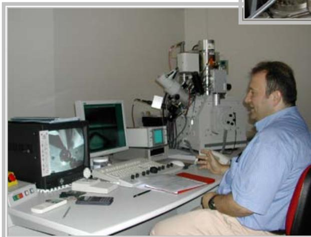
Dual beam FIB-SEM instrument (FEI STRATA DB235M) used for nanofabrication by FIB nanomachining and by electron and ion beam-induced deposition of conductive, insulating and magnetic materials from gas precursors.
