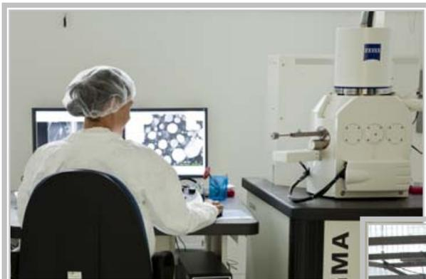
EBL system based on a field emission SEM (Zeiss SIGMA) controlled by a Raith ELPHY Quantum pattern generator.
